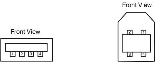
FIGURE 15–15 The front view of the two common types of USB connectors.
