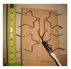
Fig.3 fractal antenna tree
