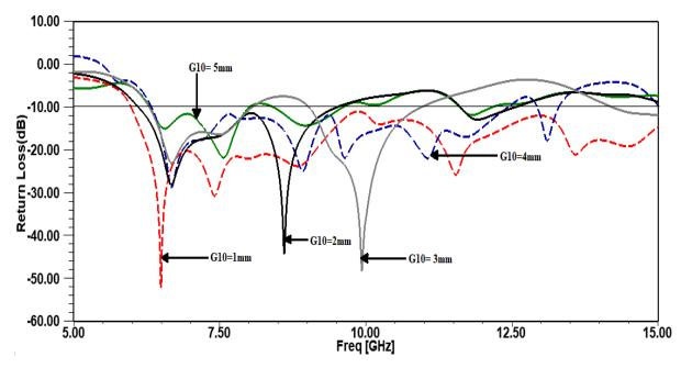
fig10. Presence of gap in the return loss
