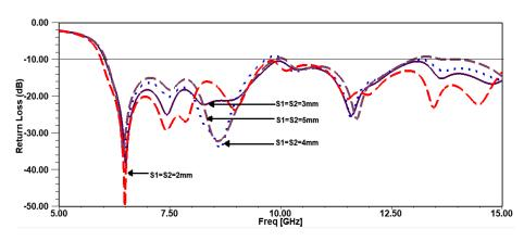
fig 9. return loss due to the presence of two split rings
