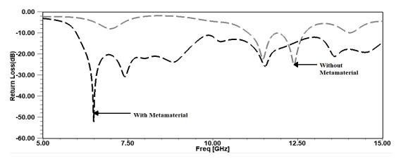
fig 8 return losses with and without the metamaterial
